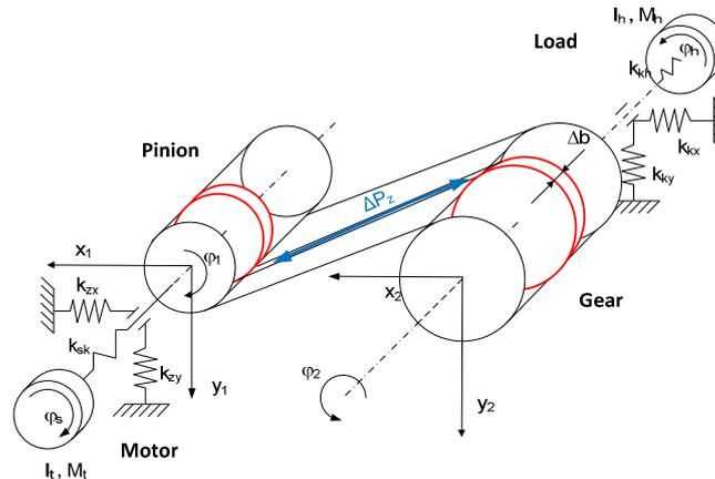
Figure 1. Simplified scheme of the simulation model of helical gear [18]
