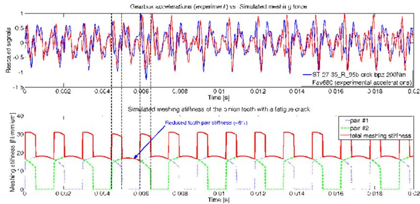
Figure 2. Comparison of gearbox acceleration recorded during the experiment and simulated meshing force for 6% reduction of stiffness on one tooth pair
