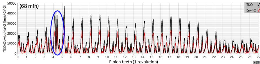
Figure 3. Comparison of squared envelope and TKEO for the acceleration signal from the 68 min. of the experiment (see Figure 2)
