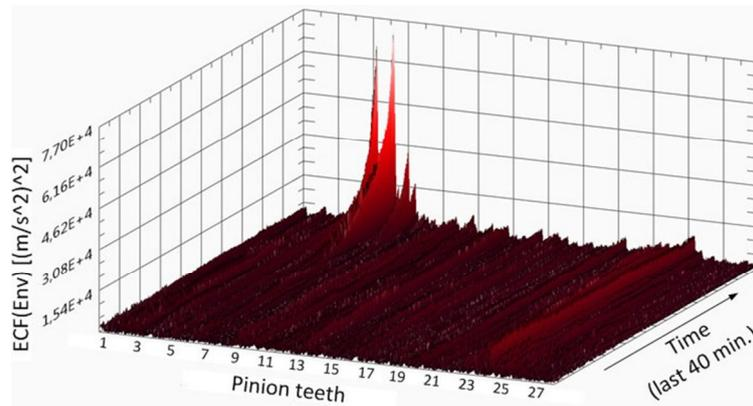
Figure 4. ECF signal for the last 40 min. of the experiment (total of 72 min.)
