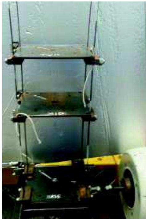
Figure 1. Time-variant three-floor building model
