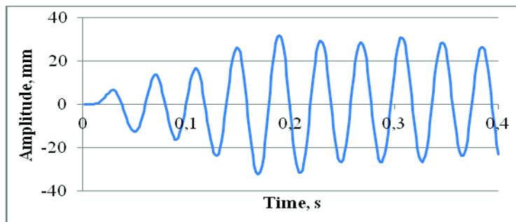
Figure 3. Transient response of the sieve for excitation frequency: 51.13 Hz
