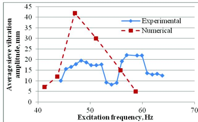
Figure 5. Effect of excitation force on sieve vibration amplitude for different excitation frequencies
