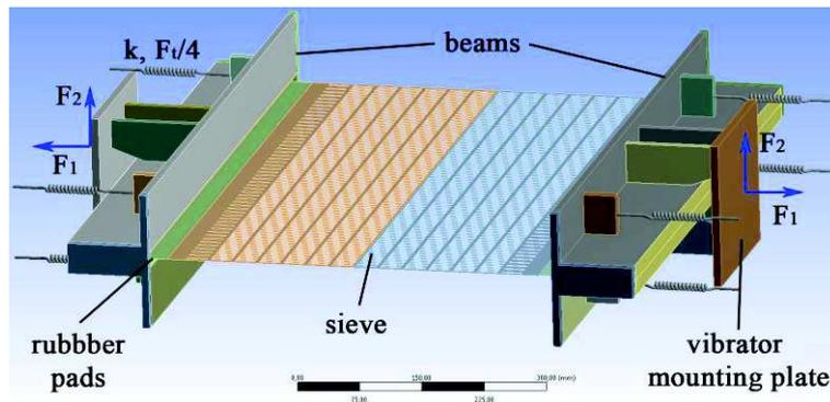
Figure 1. The simplified screen system prepared in Ansys Workbench Design Modeler
