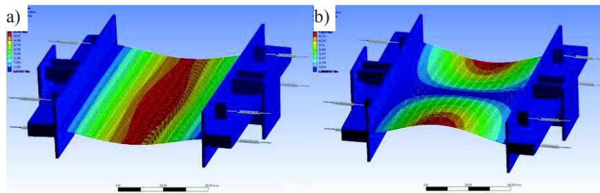
Figure 2. Free vibrations mode shapes of screen system: a) first mode; b) second mode
