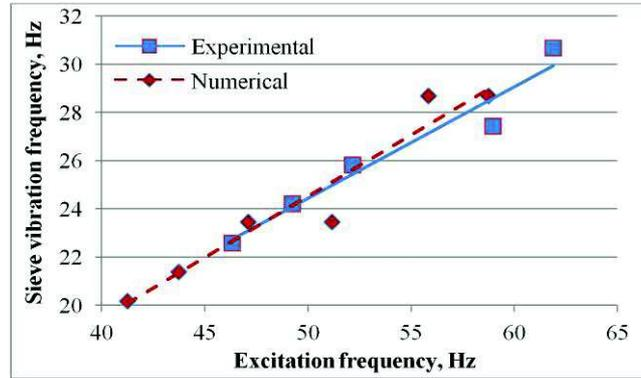
Figure 4. Effect of excitation force on sieve vibration frequency
