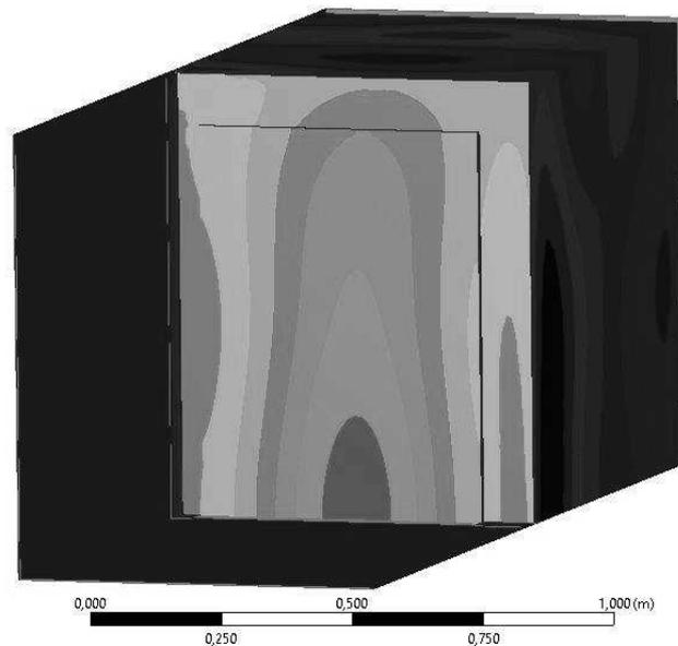
Figure 2. The calculation space with sound pressure level results for 500 Hz excitation
