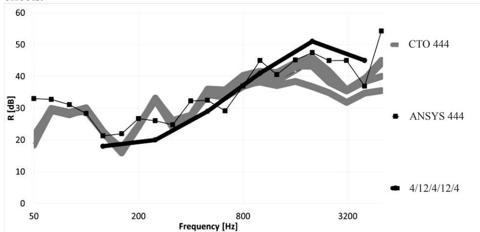
Figure 4. The comparison of numerical ANSYS 444 and experimental CTO 444 results for 4/12/4/12/4 type of window glazing
