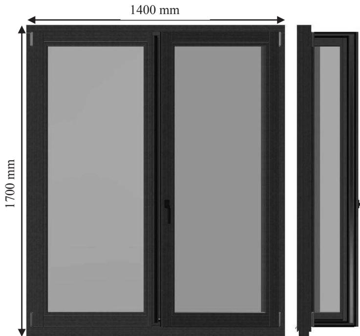
Figure 1. The CAD model of analysed window
