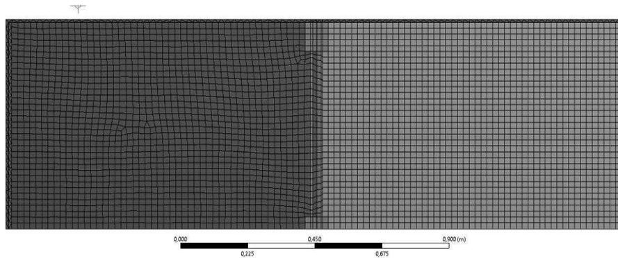
Figure 3. Geometry of the model (half-bottom view) and finite element size
