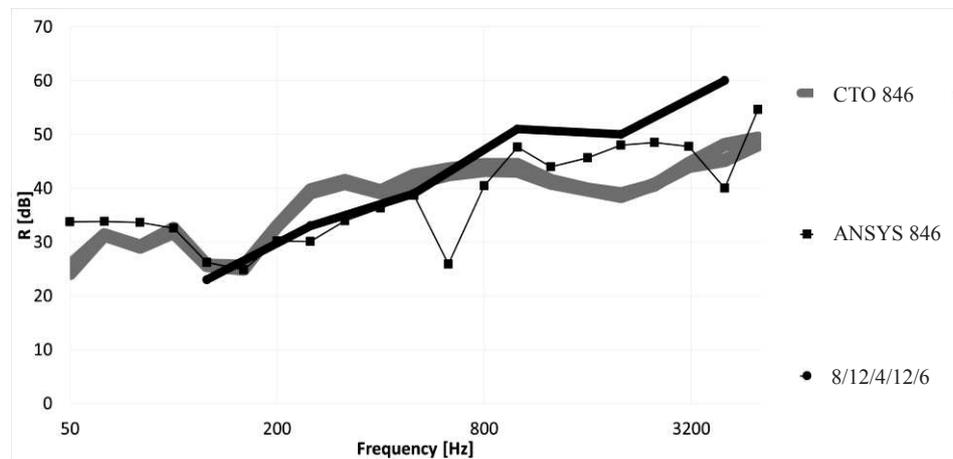
Figure 5. The comparison of numerical ANSYS 846 and experimental CTO 846 results for 8/12/4/12/6 type of window glazing
