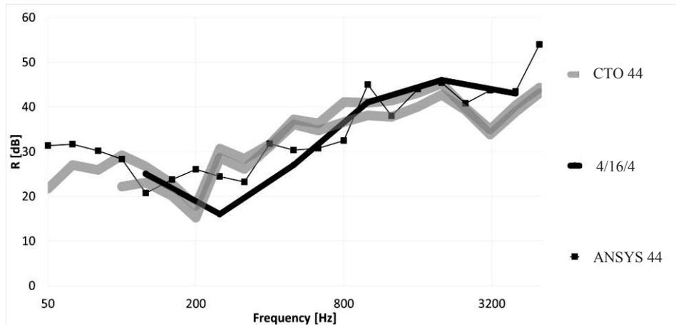
Figure 6. The comparison of numerical ANSYS 44 and experimental CTO 44 results for 4/16/4 type of window glazing
