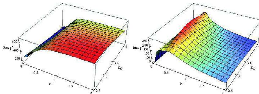
Figure 2. The dependency of the first eigenvalue ( $Re(\omega^*)$  and  $Im(\omega^*)$ ) for the cylinder on total length  $L_C$  and constructional damping  $\mu$  at  $\eta=0$ ,  $\nu=0$  and  $p=0.3$
