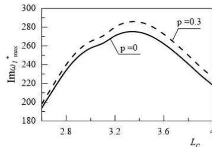
Figure 3. The relationships between the maximum values of  $Im(\omega_{max}^*)$  for the first mode of vibration in the cylinder and the extension total length  $L_C$  (for  $\eta=0$  and  $\nu=0$ )
