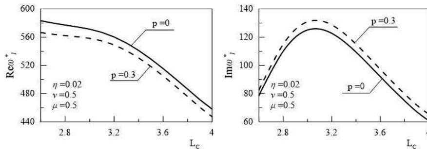
Figure 4. The dependency of the first eigenvalue ( $Re(\omega^*)$  and  $Im(\omega^*)$ ) for the cylinder on extension total length  $L_C$
