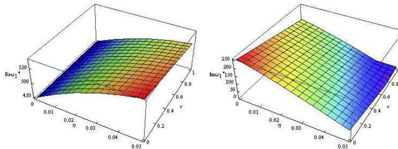
Figure 5. The dependency of the first eigenvalue ( $Re(\omega^*)$  and  $Im(\omega^*)$ ) for the cylinder on internal damping  $\eta$  and external damping  $\nu$  at  $\mu=0.5$  and  $L_C=3$
