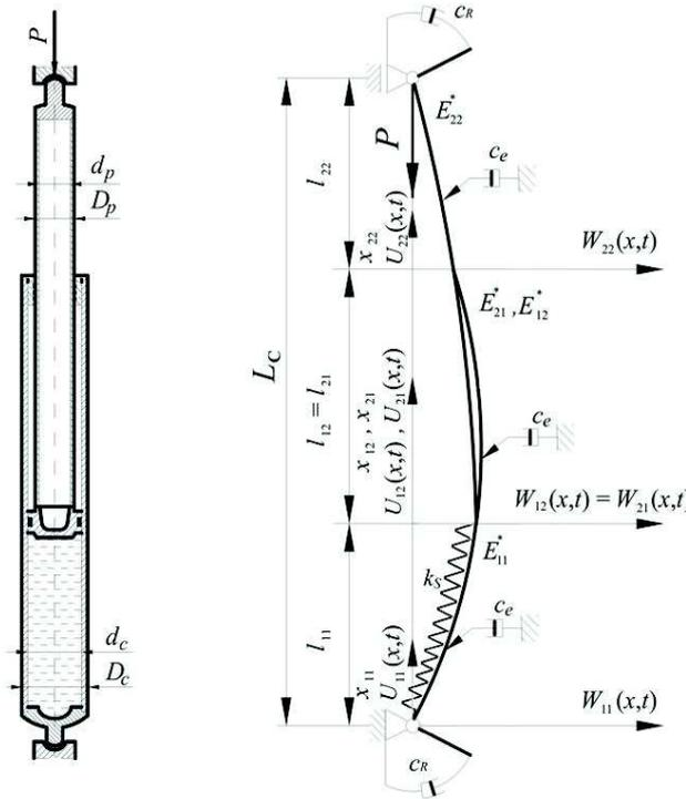
Figure 1. Diagram and beam model of a hydraulic cylinder with damping
