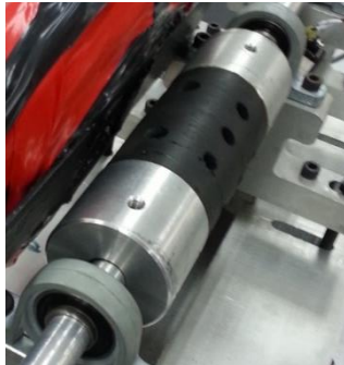
Figure 5. MRE formed in the shape of a cylinder, which was then placed inside a solenoid, as shown in item (4) in Figure 5
