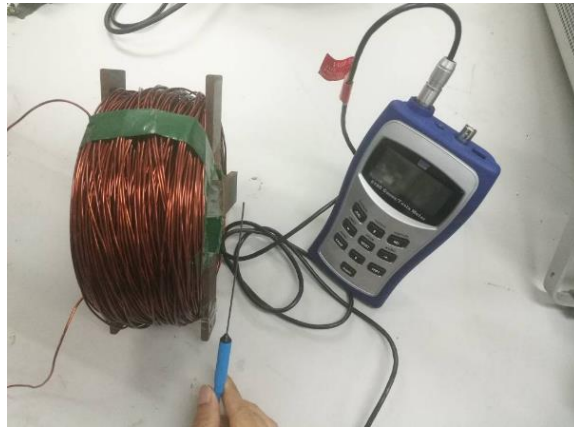
Figure 8. Measuring magnetic field using FW Bell Gaussmeter
