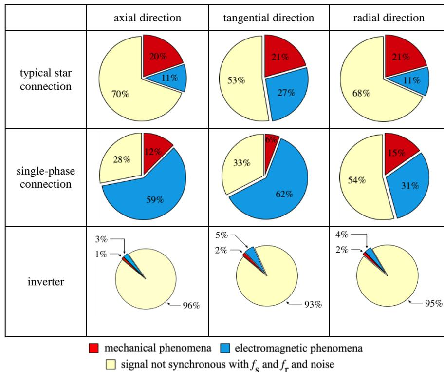
Figure 9. Summary of results of multi-synchronous decomposition of the vibration acceleration signal recorded on the front end shield of the motor
