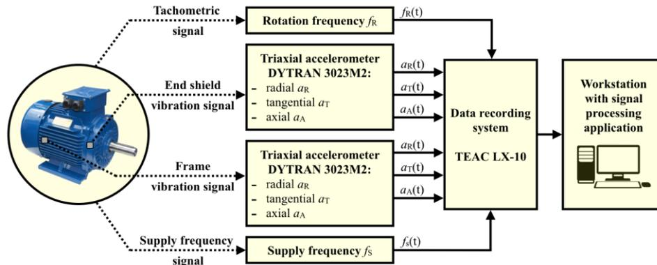
Figure 3. Diagram of the measurement chain
