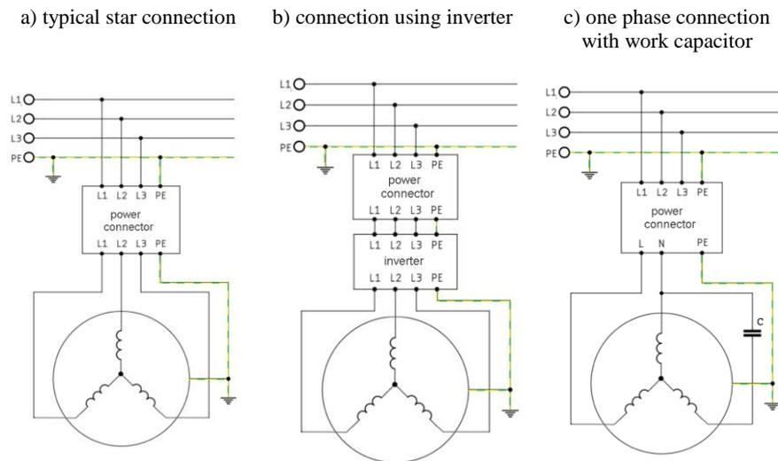
Figure 2. Power supply options of the tested AEM
