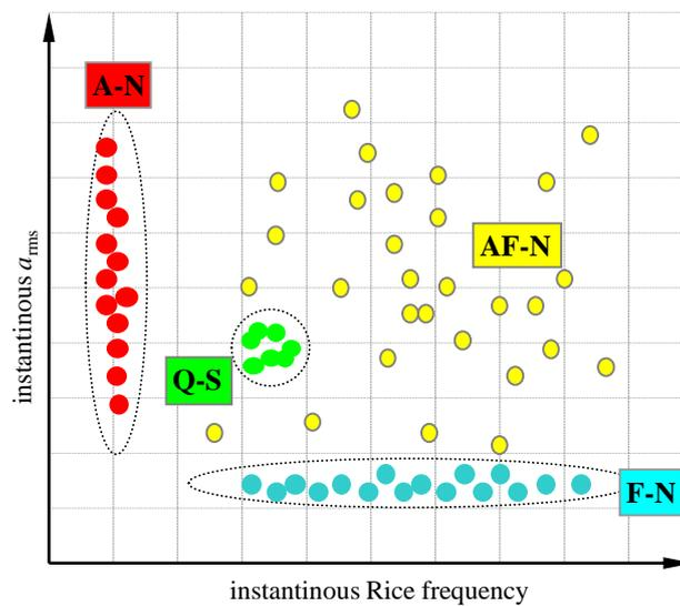
Figure 3. The idea of interpreting the results of short-time parameterisation of vibrations; a representation of various vibration signal types on the  $R_f - a_{rms}$  plane: A-N non-stationary amplitude; F-N non-stationary frequency, Q-S quasi-stationary signal, AF-F non-stationary signal in amplitude and frequency terms
