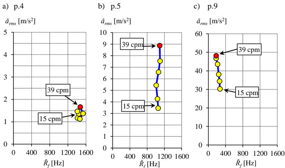
Figure 6. The change in the position of the result of the parameterisation of vibration accelerations on the  $R_f - a_{rms}$  plane resulting from the increase in machine capacity from 15 to 30 cycles per minute (cpm) a) gearmotor base b) punch guide c) cardboard bender [4]
