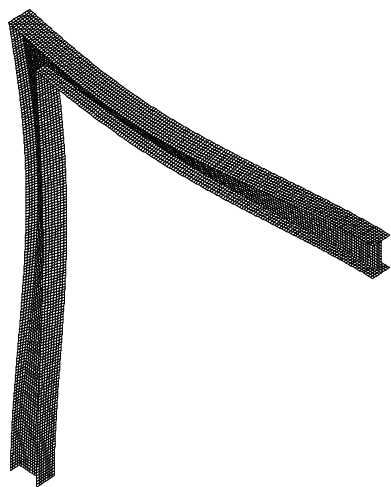
Fig. 5. Second eigenmode of the frame n_2=32.88 Hz
