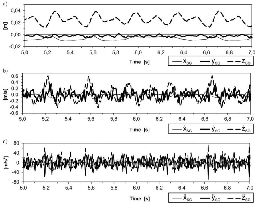
Figure 2. Boom vibration components in the intersection point of the boom longitudinal axis with the axis of rotation of cutting heads: a) displacement, b) speed, c) acceleration
