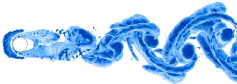
Figure 5. Unsteady flow around wall-mounted cylinder (top view) visualized with the  $\Lambda_2$  criterion
