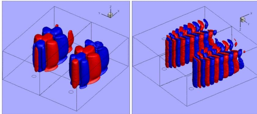
Figure 4. Real and imaginary part of modes for the flow around the wall-mounted cylinder. Left: von Karman mode, right: higher, shear-layer mode
