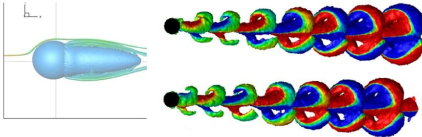
Figure 3. Steady flow around a sphere at  $Re=250$  (left). Streamlines and wake contour is shown (isosurface of  $V_x = 0$ ). Right: real (top) and imaginary (bottom) part of the dominating shedding mode visualized with the  $\Lambda_2$  criterion
