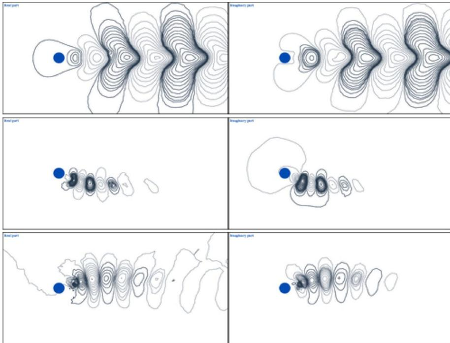
Figure 2. Real (left) and imaginary (right) part of the mode for different forcing of the flow around two-dimensional circular cylinder at  $Re = 100$
