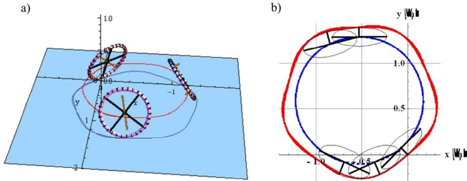
Figure 5. Unicycle wheel simulation results: a) 3D view, b) wheel – floor contact point trajectory (dashed line) and wheel centre trajectory (solid line)
