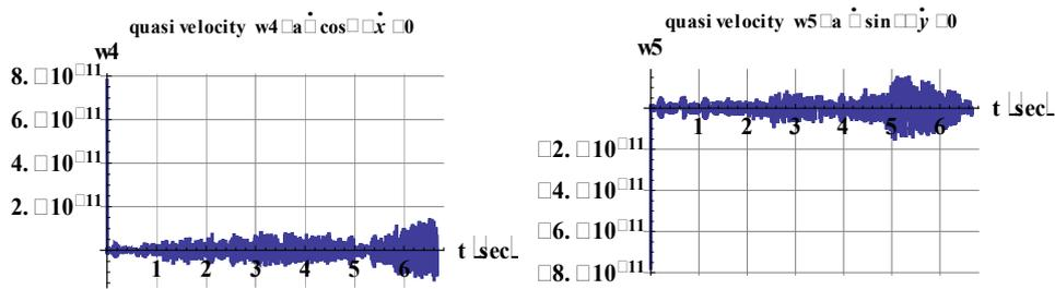
Figure 8. Constraints equations error (quasi-velocities values  $w_4$  and  $w_5$ )
