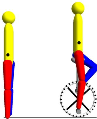
Figure 2. Average person's centre of gravity and the unicyclist's centre of gravity position
