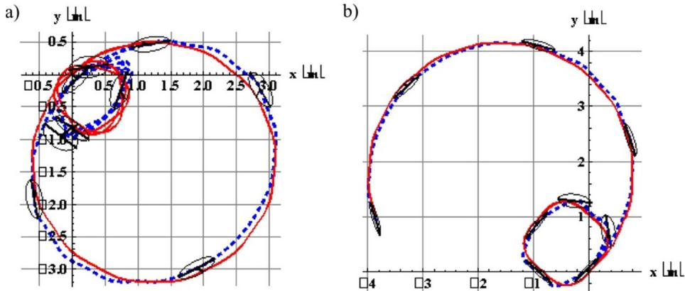
Figure 6. Comparison of contact point trajectories and wheel centre trajectory for different initial velocity ( $\dot{\varphi}$ ) and roll angle ( $\theta$ ):
