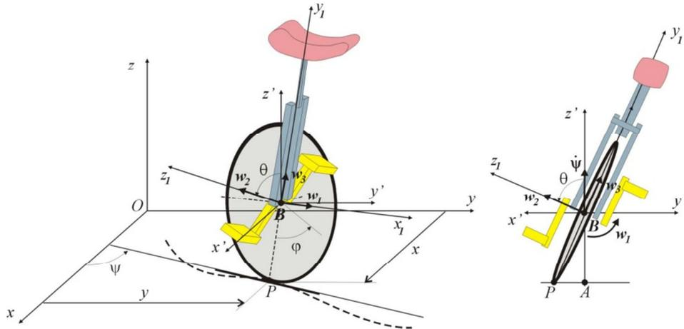
Figure 4. Model of the unicycle – without unicyclist
