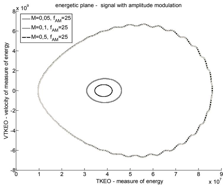
Figure 2. Signals with amplitude modulation with different depth of modulation on energetic plane
