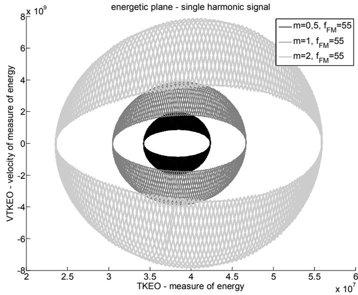
Figure 3. Signals with frequency modulation with different index of modulation on energetic plane
