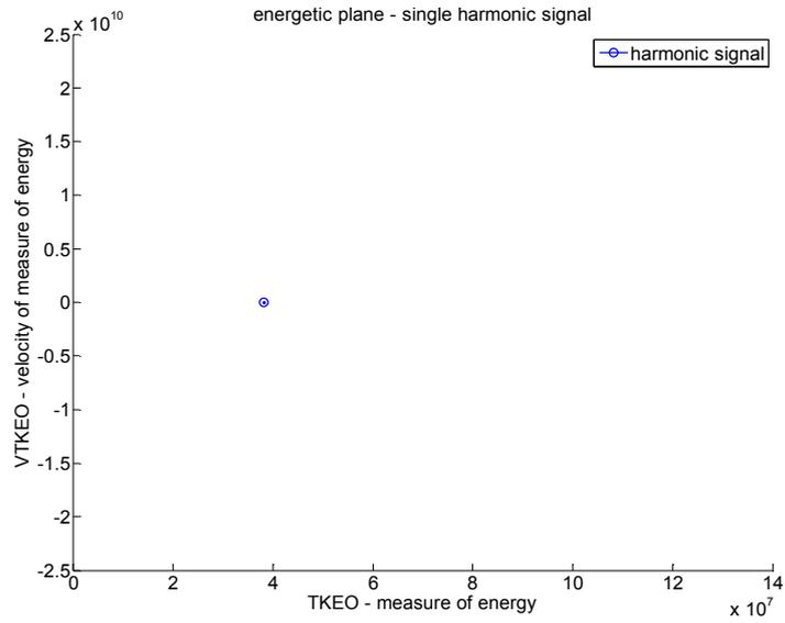
Figure 1. Single harmonic signal on energetic plane
