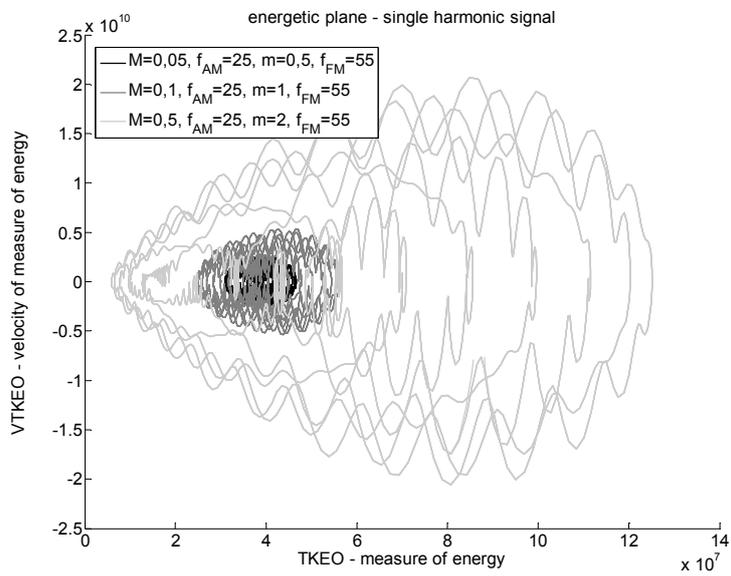
Figure 4. Signals with AM and FM modulation with different parameters of modulation on energetic plane
