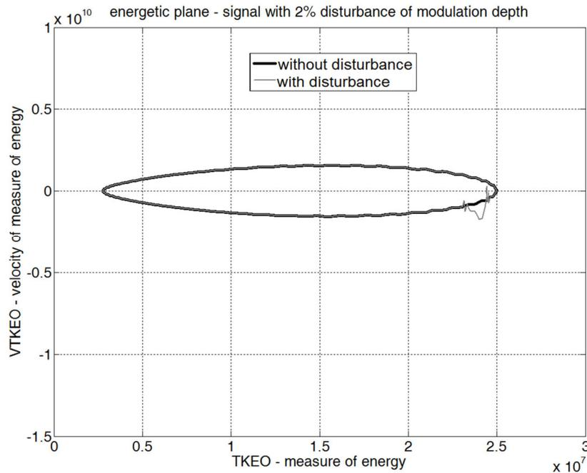
Figure 5. Signal with and without distribution of depth of AM, disturbance 2%
