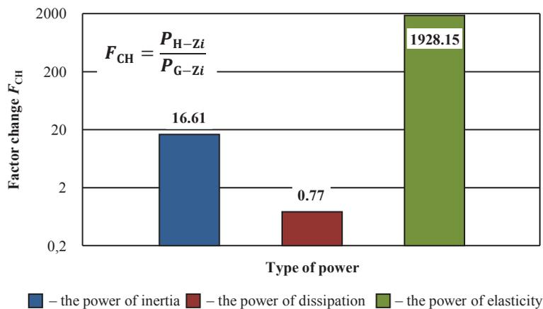
Figure 3. Quantitative comparison of three kinds of powers between the human model and the glove model for the operating frequency of the tool  $f=20$  Hz
