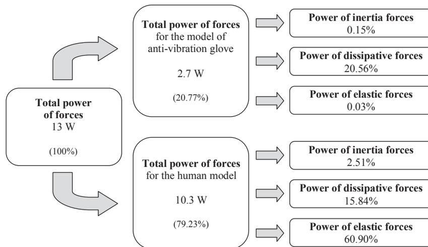
Figure 2. The structural power distribution of forces for the human model and the glove model [6] for the operating frequency of the tool  $f = 20$  Hz
