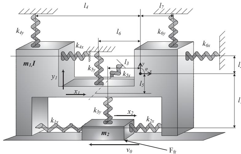
Figure 1. The considered 4-DOF model with dry friction
