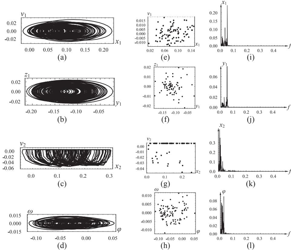
Figure 2. Phase portraits (a,b,c,d), Poincaré sections (e,f,g,h) and PSDs (i,j,k,l) for  $v_0 = 0.005$  in time interval  $\tau \in (20000, 22000)$
