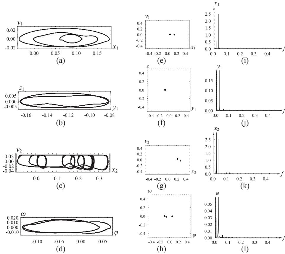
Figure 3. Phase portraits (a,b,c,d), Poincaré sections (e,f,g,h) and PSDs (i,j,k,l) for  $v_0 = 0.025$  in time interval  $\tau \in (20000, 22000)$
