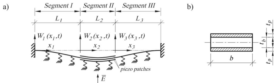
Figure 1. Scheme of clamped-clamped beam resting on elastic Winkler foundation with two piezoelectric patches colocally mounted along the central segment (a), piezosegment cross-section (b)
