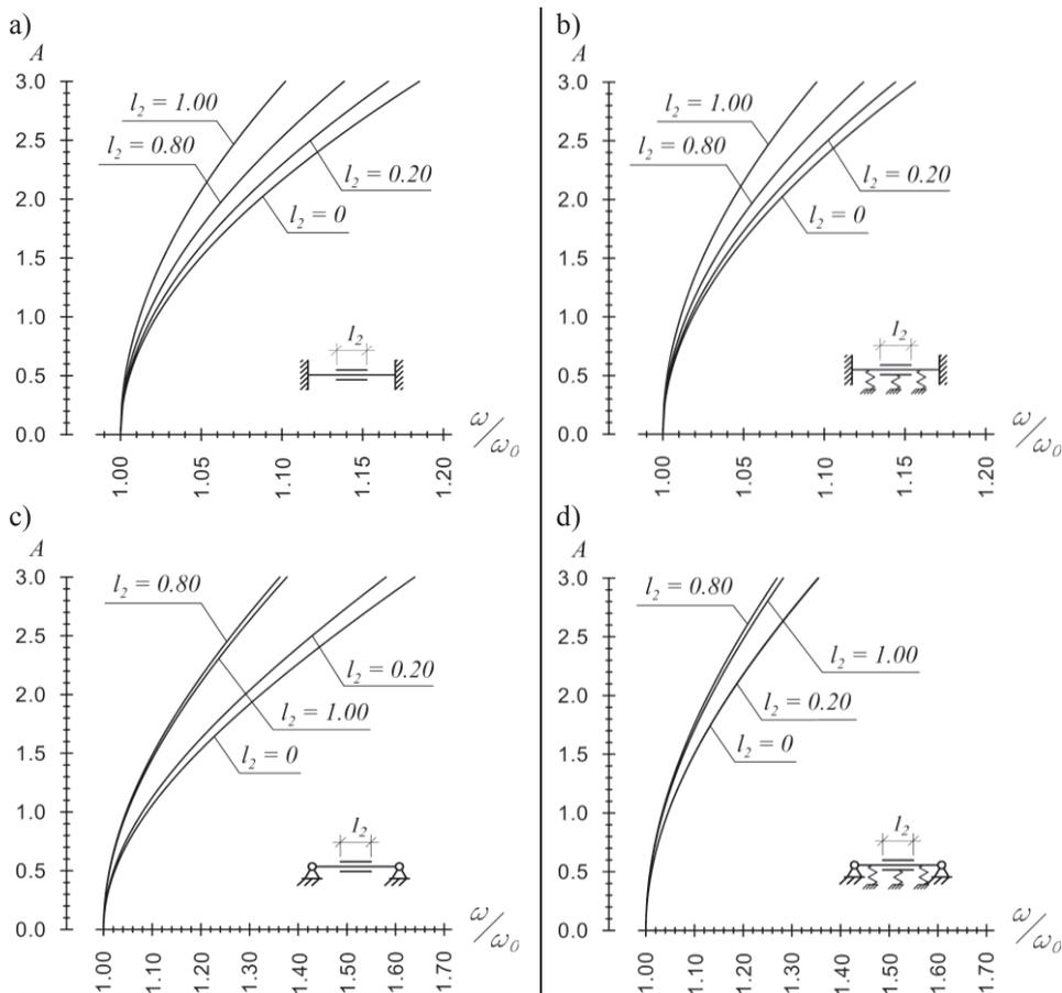
Figure 2. The influence of piezosegment length on amplitude – non-linear frequency relationship in clamped-clamped (a, b) and pinned-pinned (c, d) beams; remaining parameters: Winkler elastic foundation modulus  $\beta = 0$  (a, c),  $\beta = 100$  (b, d)
