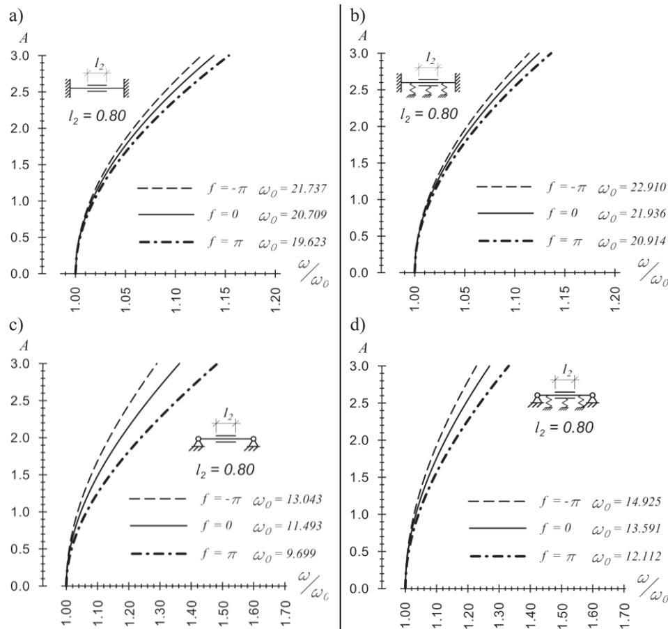
Figure 3. The influence of piezoelectric actuation on the amplitude-non-linear frequency relationship for clamped-clamped (a, b) and pinned-pinned (c, d) beams; remaining parameters: Winkler elastic foundation modulus  $\beta = 0$  (a, c),  $\beta = 100$  (b, d)
