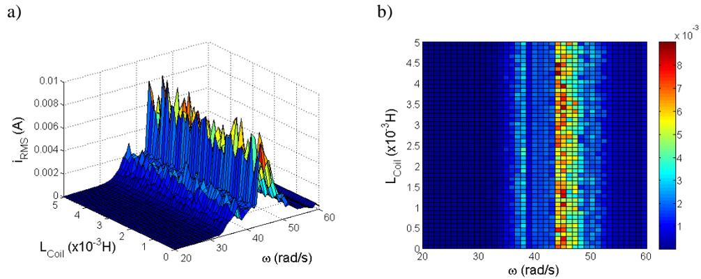
Figure 2. 3D characteristics  $i_{RMS}$  versus  $L_{Coil}$  and  $\omega$  (a), and top view (b)
