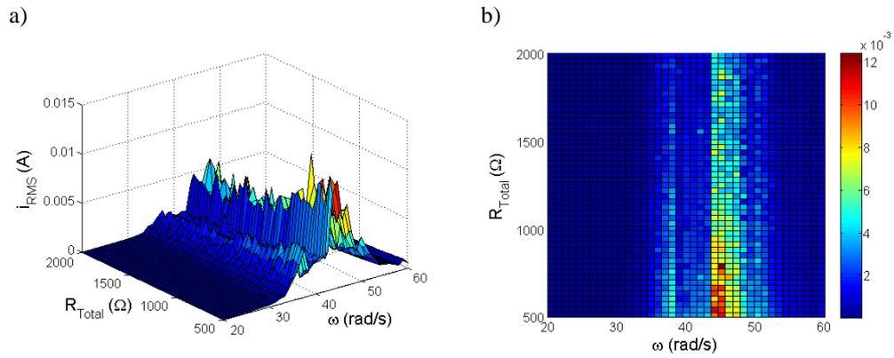
Figure 3. 3D characteristics  $i_{RMS}$  versus  $R_{Total}$  and  $\omega$  (a), and top view (b)
