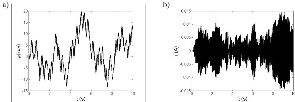
Figure 6. Time series of angle  $\varphi$  (a) and current  $i$  (b), for  $\omega=45\text{rad/s}$
