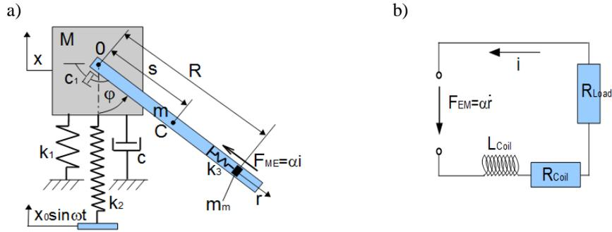
Figure 1. Model of a mechanical (a) and electrical (b) parts of the system
