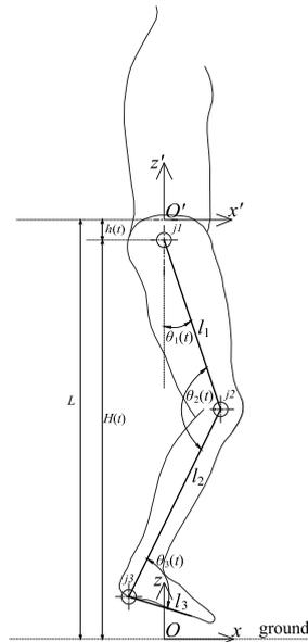
Figure 3. Biomechanical model of the human lower extremity
