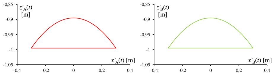
Figure 5. Phase trajectories of the joint  $j3$  in the local coordinate system  $O'x'z'$
