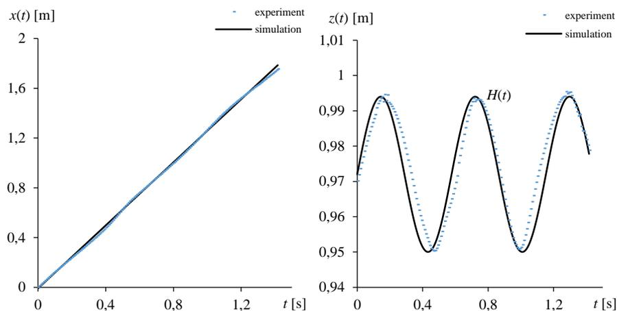
Figure 7. Experimental vs. numerical fluctuations of position of the joint  $j1$  in the forward direction (left) and the vertical direction (right)
