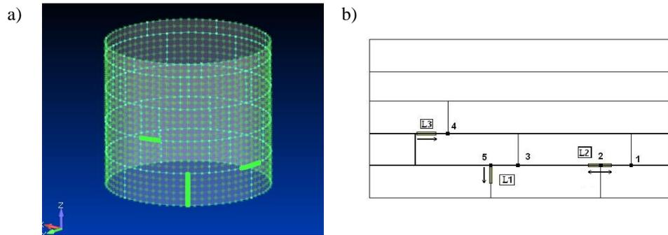
Figure 1. Discrete model of vertical weld-fabricated tank with cracks (a) and scheme of cracks location and the places of sensors installation (b)
