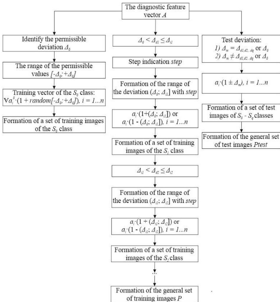
Figure 2. Algorithm of formation of training and test sets of diagnostic feature vectors
