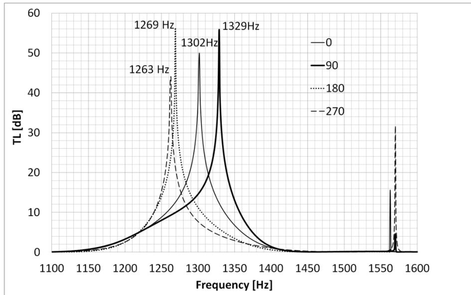
Figure 5. Transmission loss for acoustical systems with helicoidal resonator with  $s/d = 1.976$  and 90 degree duct elbow for four types of degrees of rotation
