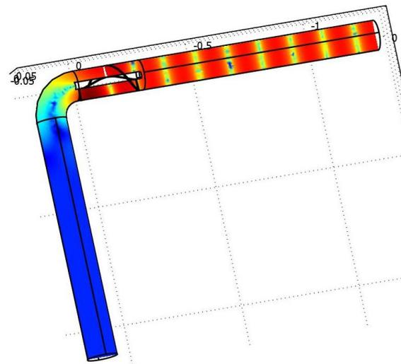
Figure 3. Sound pressure level distribution for 180 degree of rotation of 90 degree elbow and helicoidal resonator for the resonance frequency  $f = 1270$  Hz: highest dB levels – dark red colors, lowest dB levels – blue colors
