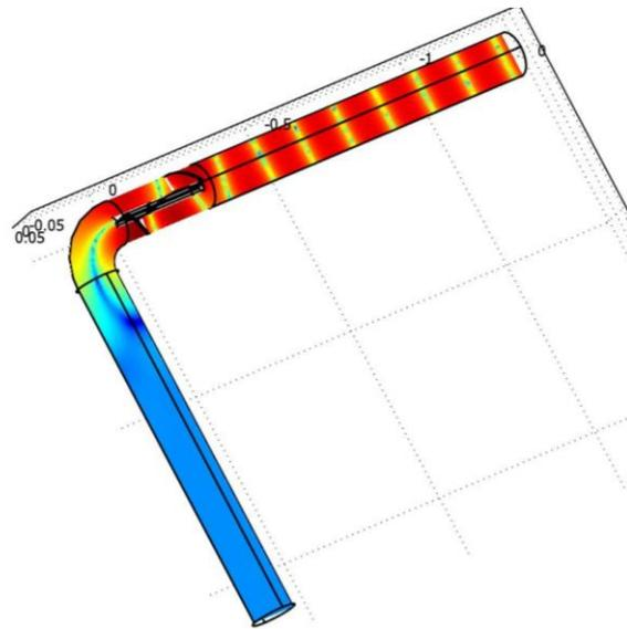
Figure 2. Sound pressure level distribution for 90 degree of rotation of 90 degree elbow and helicoidal resonator for the resonance frequency  $f = 1330$  Hz: highest dB levels – dark red colors, lowest dB levels – blue colors
