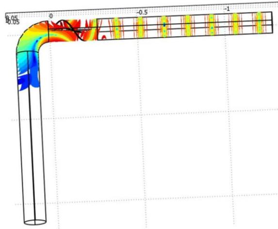
Figure 4. Sound pressure level distribution for 270 degree of rotation of 90 degree elbow and helicoidal resonator for the resonance frequency  $f = 1263$  Hz: highest dB levels – dark red colors, lowest dB levels – blue colors
