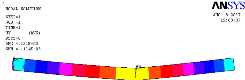
Figure 5. Zero frequency deflection plot of a cracked simply supported beam;
