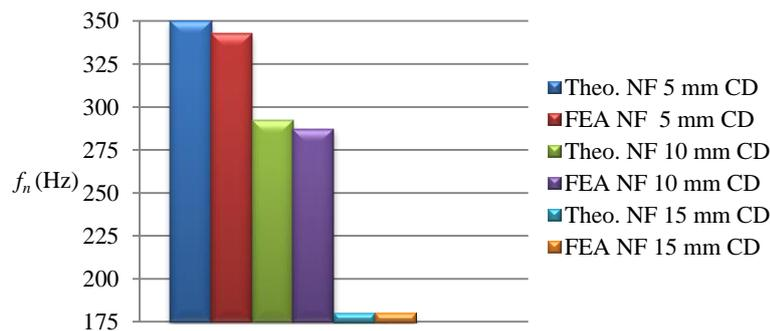
Figure 9. Comparison of first bending natural frequency of a simply supported beam with three-edged cracks:  $L_1/L = 0.278$ ;  $L_2/L = 0.556$ ;  $L_3/L = 0.834$
