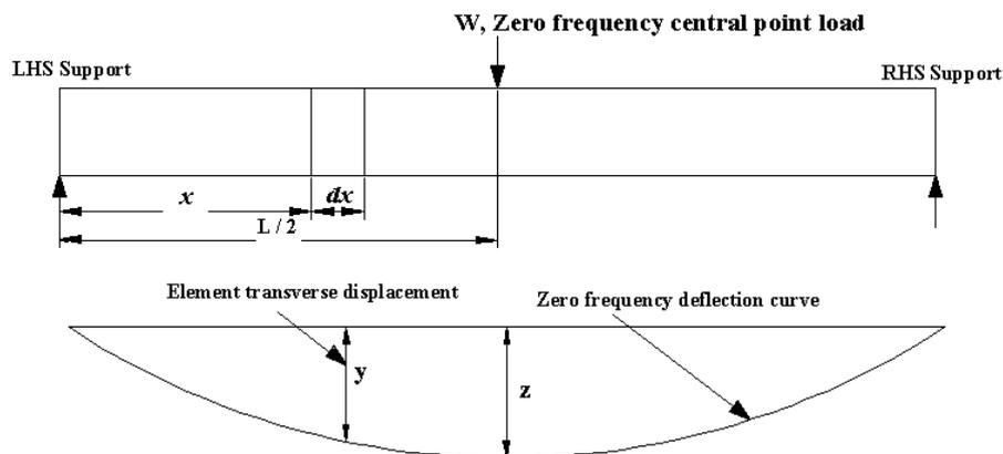
Figure 1. A schematic diagram of a simply supported beam subjected to zero frequency central point load
