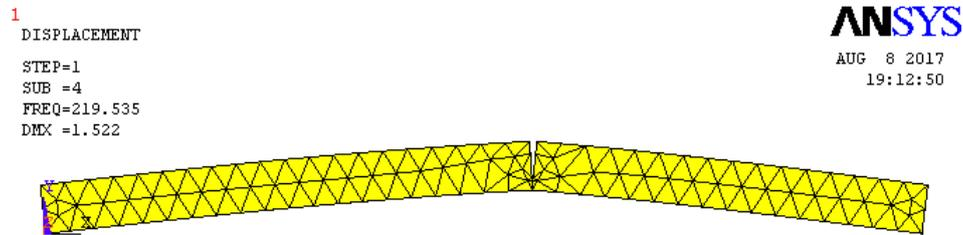
Figure 6. Natural frequency plot of a cracked simply supported beam;
