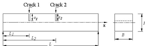
Figure 3. A schematic diagram of a cracked simply supported beam with two cracks
