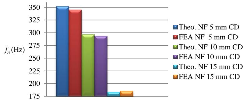
Figure 8. Comparison of first bending natural frequency of a simply supported beam with two-edged cracks:  $L_1/L = 0.278$ ;  $L_2/L = 0.556$
