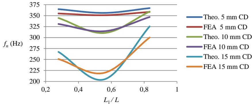
Figure 10. Variation of natural frequency with crack location ratio for single-edged cracked cases
