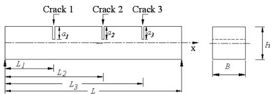
Figure 4. A schematic diagram of a cracked simply supported beam with three cracks
