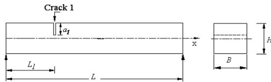
Figure 2. A schematic diagram of a cracked simply supported beam with single crack
