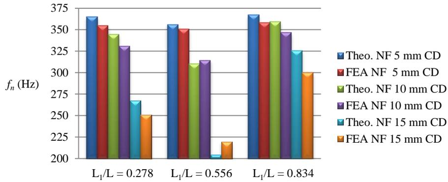
Figure 7. Comparison of first bending natural frequency of a simply supported beam with single-edged crack for 100 mm, 200 mm and 300 mm crack location
