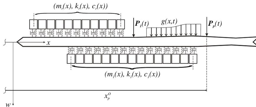
Figure 1. Beam with the system of distributed mass dampers
