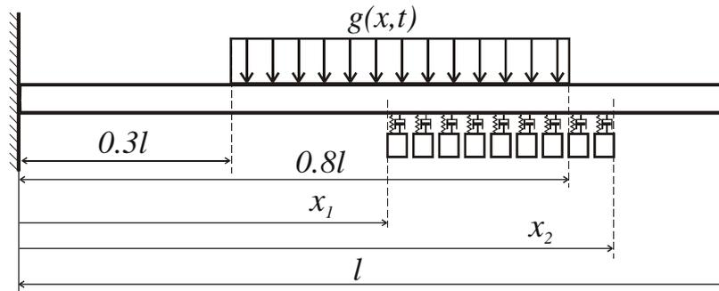
Figure 2. Beam with the attached tunable mass damper
