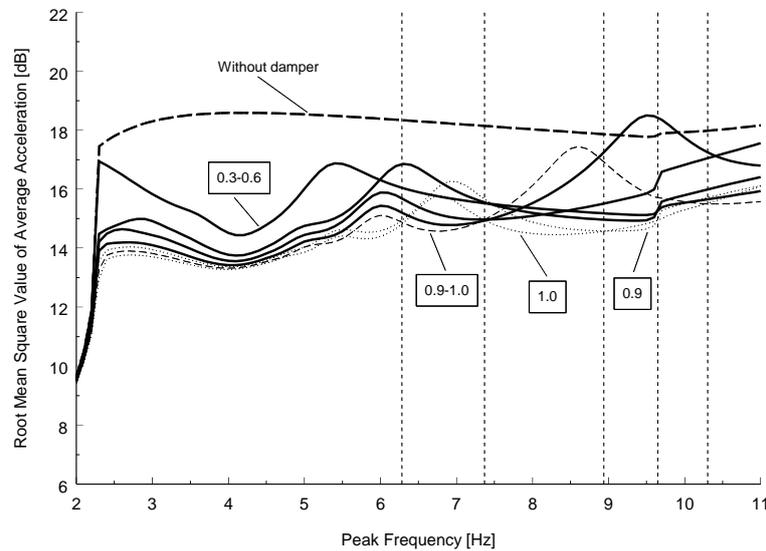
Figure 3. Root mean square values of the average beam acceleration vs. peak frequency. The damper is tuned exactly to the peak frequency of the power spectral density with parameter  $\beta = 1.0$ . Damping ratio of the damper equals to 0.1
