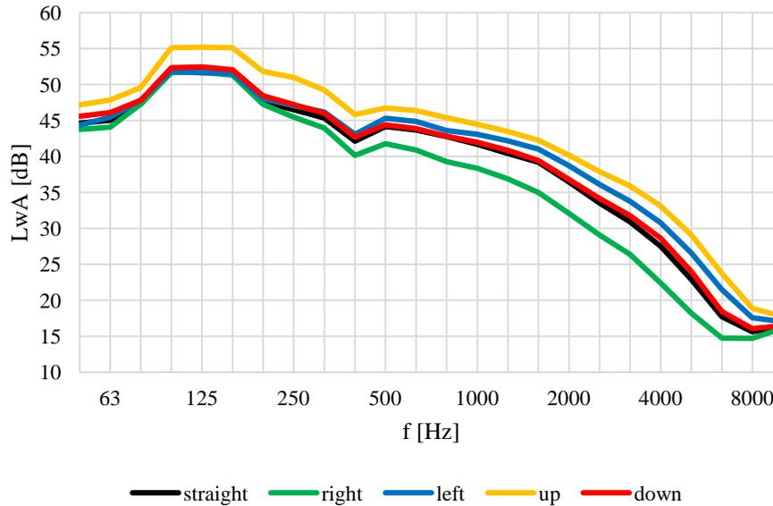
Figure 6. Acoustic power level spectrum for different blade settings with diffuser B and volume flow 1000 m<sup>3</sup>/h
