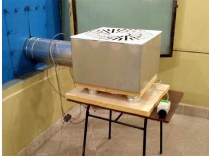
Figure 4. Plenum box with swirl diffusers under test
