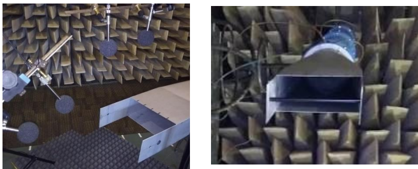
Figure 1. The construction of test stand with outflow to anechoic room and microphones
