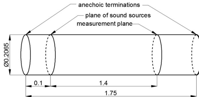
Figure 1. Geometry of the waveguide (dimensions in [m])
