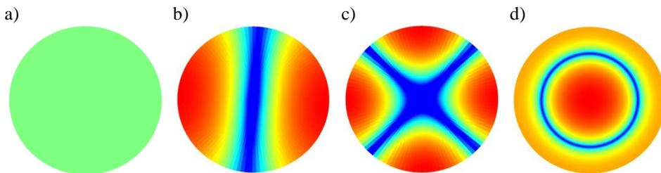
Figure 6. Theoretical shape functions of modes: a) mode (0,0), b) mode (1,1), c) mode (2,1), d) mode (0,1)
