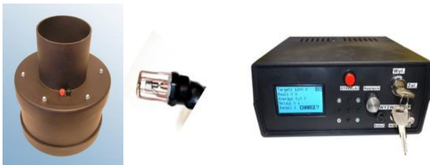
Figure 1. Microflown low frequency omnidirectional source (left) [7] and spark gap sound source for scale modelling [8]
