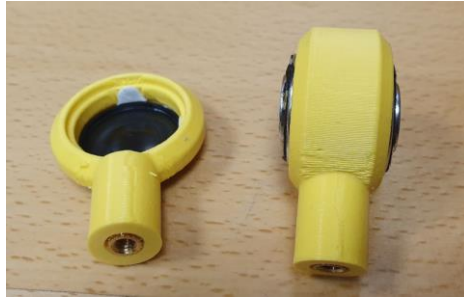
Figure 5. Test samples for the experiment – single speaker (left) and isobaric in-phase (right)
