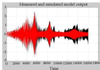
Figure 6. Identification results for chirp signal of 20-500 Hz
