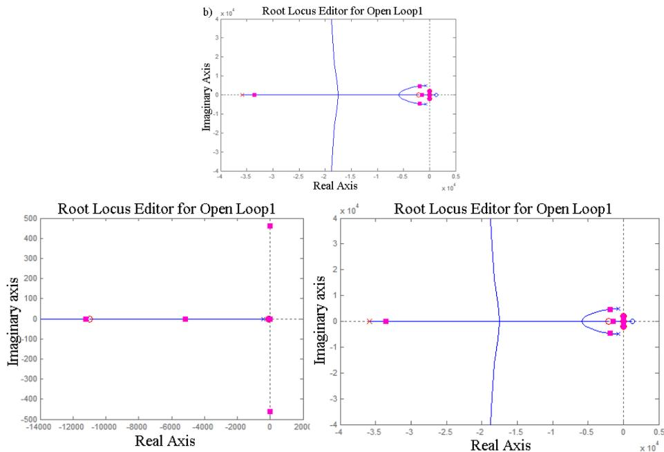
Figure 8. Location of zeros and poles of the system: a) identified 73 Hz, b) identified 315 Hz, c) identified chirp
