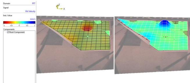
Figure 3. Resonant model shape. Maximum velocity amplitude
