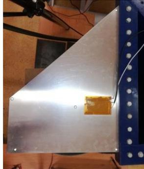
Figure 1. Research object with attached MFC sensor/actuator
