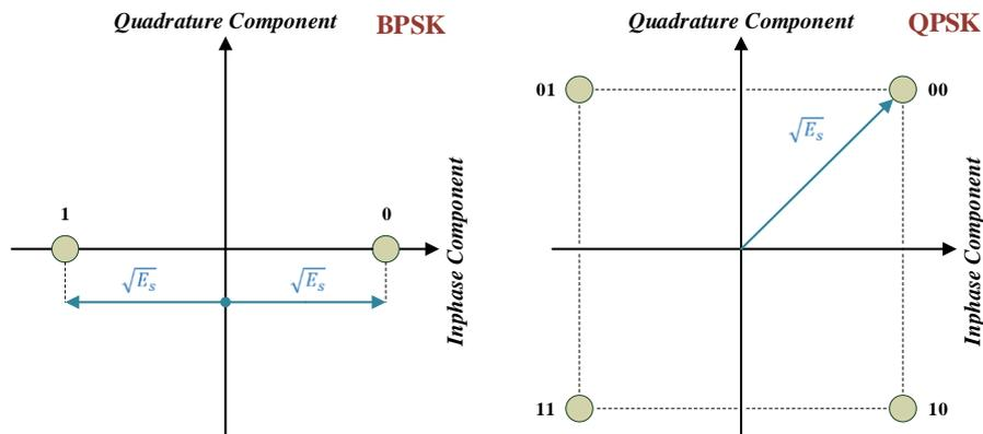
Figure 1. Space constellation diagrams for BPSK and QPSK
