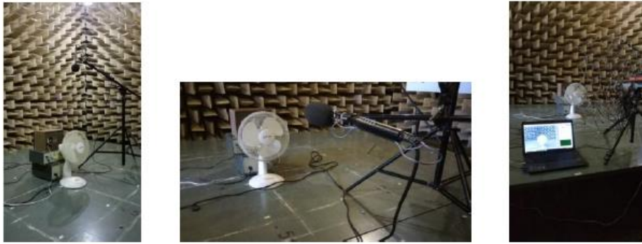
Figure 1. System of noise source composed from loudspeaker and fan, and measurement with sound analyser (on the left), intensity probe (in the centre) and acoustic camera (on the right) are being made
