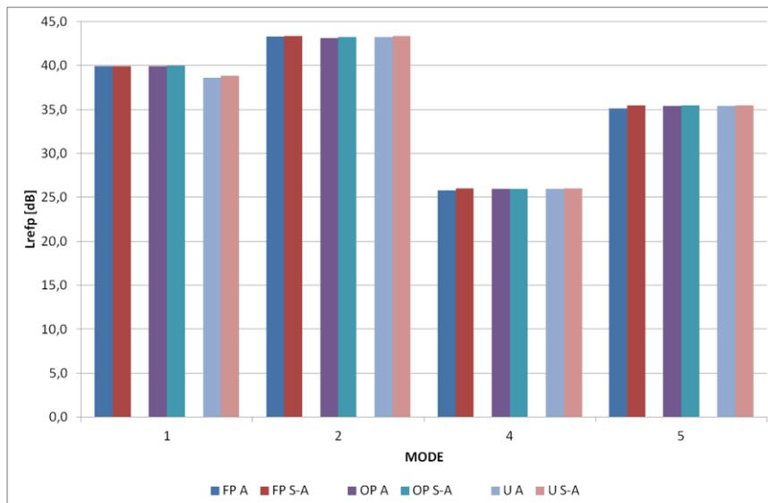
Figure 3. Comparison of vibration level reduction when recalculated to the  $L_{redf}$ ; the FP stands for when using the whole plate as a sensor; OP then using sensor placed on the diagonal in the upper part of the plate; U when using sensor placed under the actuator; A is the “standard” actuator and S-A is the sensor-actuator
