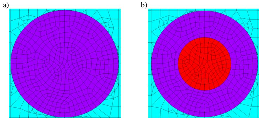
Figure 2. Disc based actuator a) when used as a standard actuator, b) when simulating a sensor-actuator
