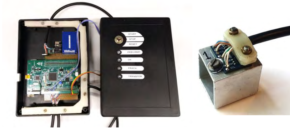
Figure 1. The controller board in its casing (left) and the MEMS accelerometer mounted on a piece of rectangular pipe (right)
