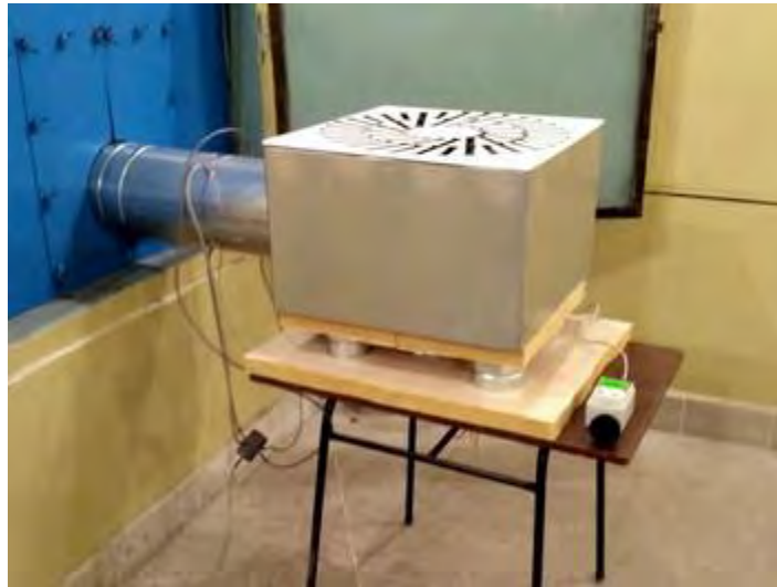
Figure 4. Plenum box with swirl diffusers under test
