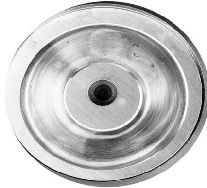
Figure 2. Demonstration of deflected swashplate wear
