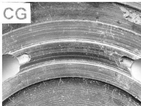
Figure 3. View of flow micro-conduits on worn valve plate
