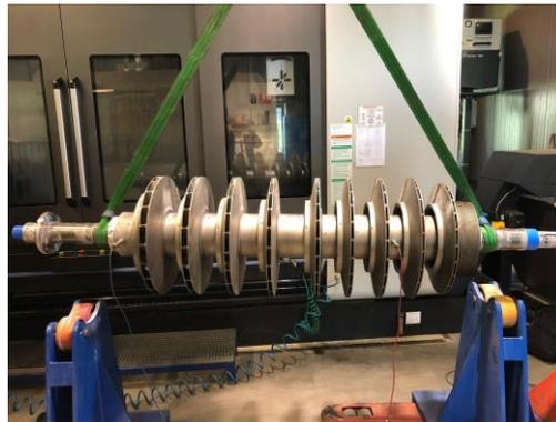
Figure 3. Free-hanging rotor of the compressor during natural vibration measurements for numerical model tuning
