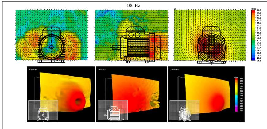
Figure 5. Diagnosis of local sources of noise generated (for  $f = 100$  Hz) by elements of an operating electric motor
