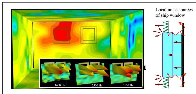
Figure 4. Searching for local noise sources in the ship's cabin using the acoustic imaging
