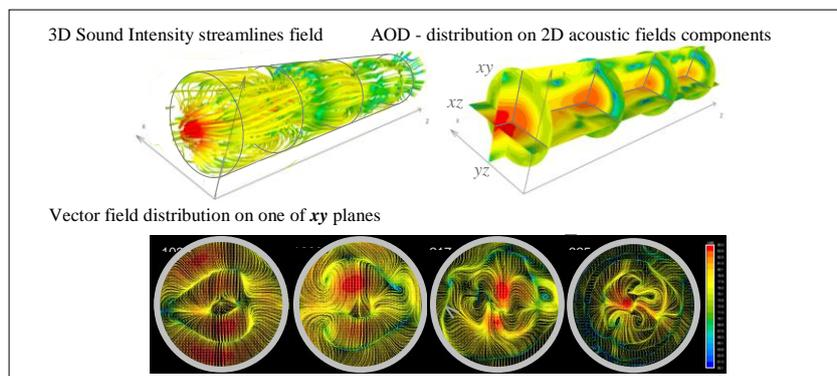
Figure 2. SI-AOD - distribution of vectors acoustic flow field inside circular duct as a function of space, frequency and amplitude
