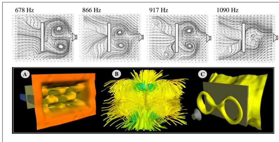
Figure 1. Sound intensity wave distribution around hard rectangular plate (for some selected frequencies): 2D intensity map with vectors (arrows) and SI, 3D shape of wave (A) and SI streamlines in the rear side of plate (B), SI isosurface in the front and rear side (C)
