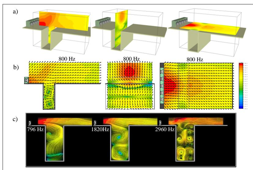
Figure 3. SI flow field for the loudspeaker line array system radiated over a flat plate with rectangular deep cavity: a) - intensity orthogonal maps;  $yz$ ,  $xy$ ,  $xz$  plane, b) – vectors distributions, c) – characteristic Rossiter modes in the cavity influence on the main flow
