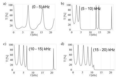
Figure 4. Transmission for the best found structures for each band a) 0 kHz – 5 kHz, b) 5 kHz – 10 kHz, c) 10 kHz – 15 kHz, a) 15 kHz – 20 kHz
