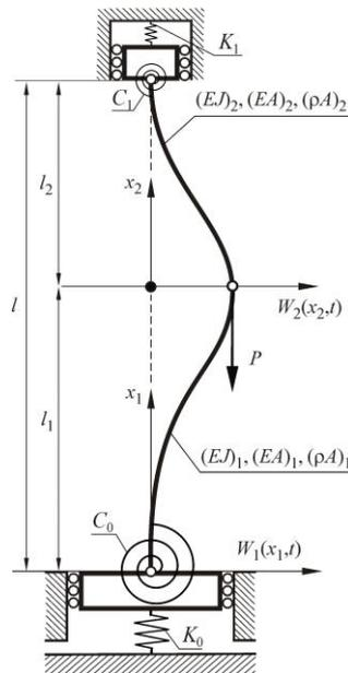
Figure 1. Physical model of considered column
