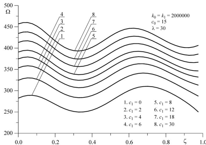
Figure 3. The relationship between natural vibration frequency  $\Omega$  and the rotational springs stiffness  $c_0$  and  $c_1$ , at different points of external load application  $\zeta$  taking into account the parameters:  $k_0 = k_1 = k$ ;  $c_0 = 15$ ;  $\lambda = 30$
