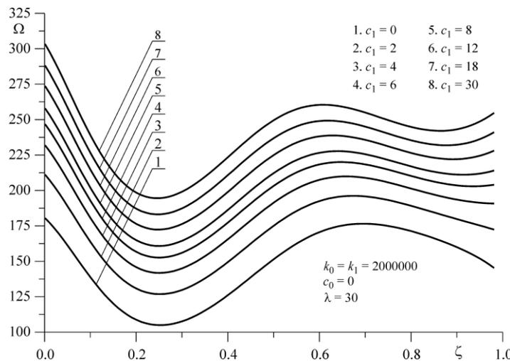
Figure 2. The relationship between natural vibration frequency  $\Omega$  and the rotational springs stiffness  $c_0$  and  $c_1$ , at different points of external load application  $\zeta$  taking into account the parameters:  $k_0 = k_1 = k$ ;  $c_0 = 0$ ;  $\lambda = 30$
