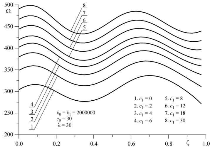
Figure 4. The relationship between natural vibration frequency  $\Omega$  and the rotational springs stiffness  $c_0$  and  $c_1$ , at different points of external load application  $\zeta$  taking into account the parameters:  $k_0 = k_1 = k$ ;  $c_0 = 30$ ;  $\lambda = 30$
