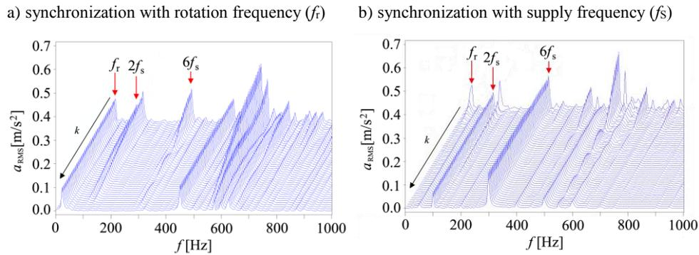
Figure 5. Changes in the spectral composition of vibration acceleration signals averaged synchronously; process synchronized with the supply frequency  $f_s$  and rotational frequency of the rotor  $f_r$  ( $k$  - subsequent iterations of synchronous averaging)
