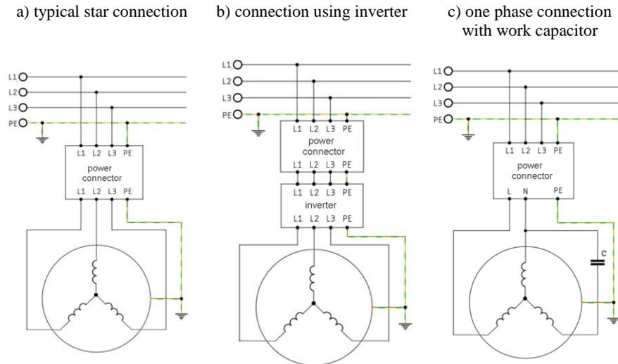
Figure 2. Power supply options of the tested AEM
