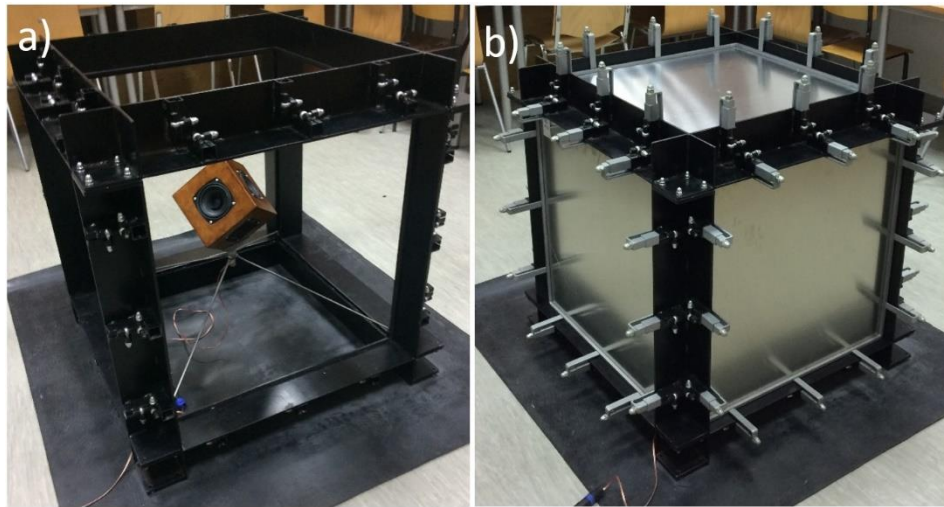
Figure 1. View of the enclosure: a) steel frame without walls and with an omnidirectional sound source, b) enclosure with walls of mineral wool-aluminium composition
