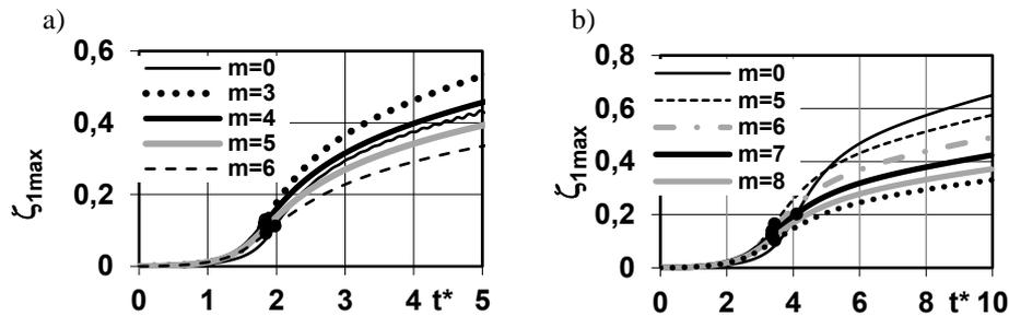
Figure 2. Time histories of deflections of FDM plate model with viscoelastic core: a)  $G_2=5$  MPa, b)  $G_2=15.82$  MPa depending on mode  $m$
