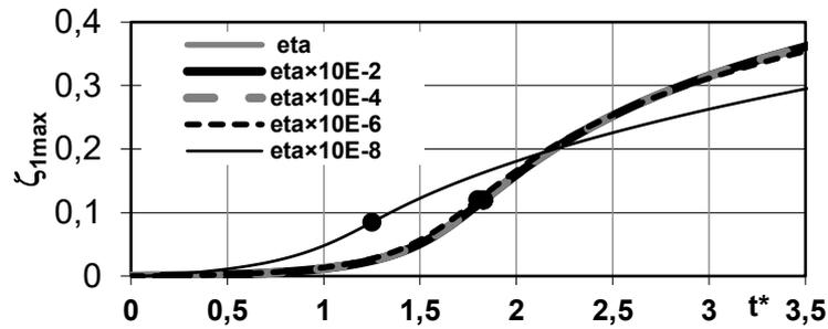
Figure 4. Time histories of deflections of FDM plate model with viscoelastic core  $G_2=5$  MPa depending on viscosity parameter  $\eta'$  (eta)
