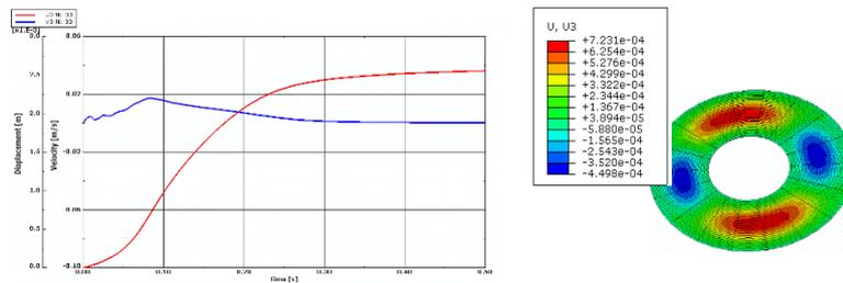
Figure 5. Time histories of deflection and velocity of deflection and buckling mode  $m=2$  of FEM plate model with viscoelastic core  $G_2=5$  MPa
