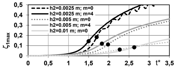
Figure 3. Time histories of deflections of FDM plate model with viscoelastic core  $G_2=5$  MPa depending on core thickness  $h_2$
