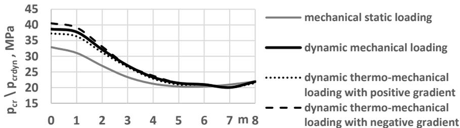
Figure 6. Distribution of values of static  $p_{cr}$  and dynamic  $p_{crdyn}$  loads for FDM plates SC-SC with viscoelastic core  $G_2=5$  MPa for two temperature fields versus buckling mode  $m$
