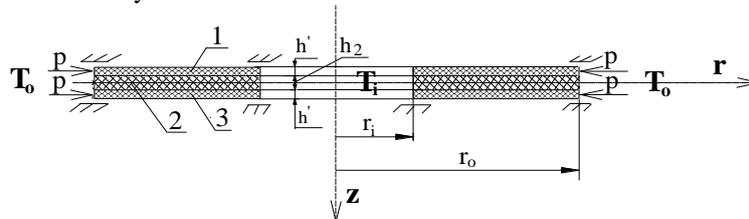
Figure 1. Scheme of three-layered annular plate composed of facings (layers 1,3) and core (layer 2) loaded with compressive stress  $p$  and subjected to axisymmetrical temperature field  $T_i, T_o$
