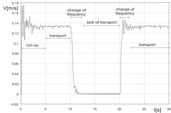
Figure 8. The feed transportation velocity
