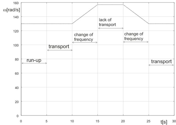
Figure 5. The angular velocity of vibrators
