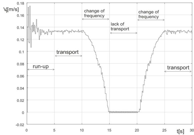
Figure 6. Transport velocity of the feed
