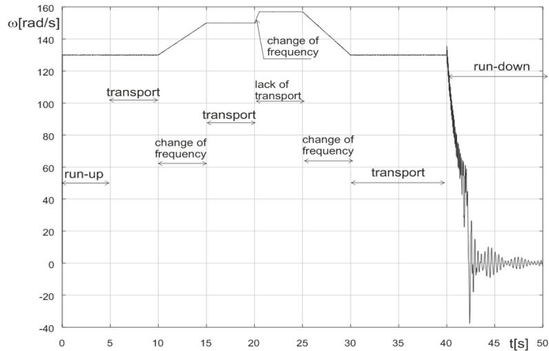
Figure 9. The angular velocity of the excitation
