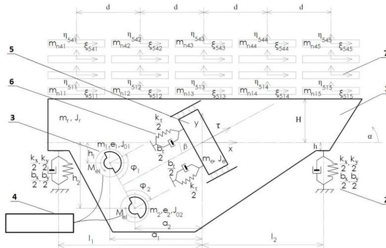
Figure 1. Scheme of the conveyor loaded with feed material - according to the invention
