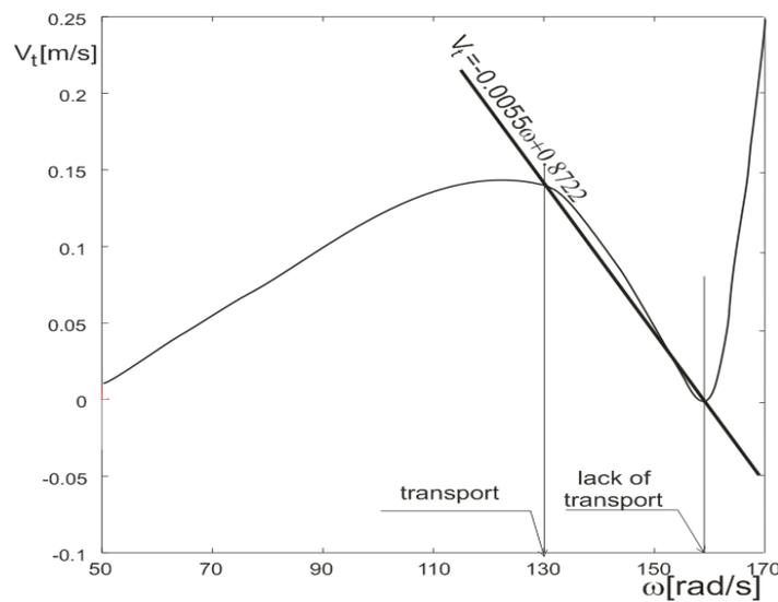
Figure 4. Transport velocity as a function of the excitation frequency
