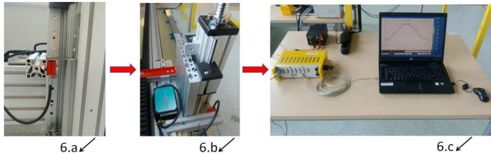
Figure 6. Flow chart of the connections between individual elements of the measurement site.
