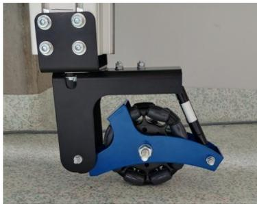
Figure 7. View of the vertical column with the suspension attached
