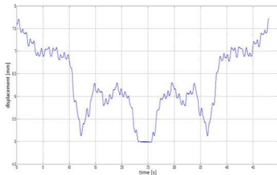
Figure 8. Course of the measured displacement of the column while driving
