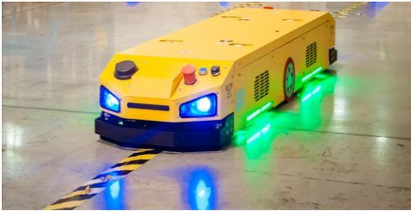
Figure 1. AGV E01 tractor type [own photo: Etisoft Smart Solutions Sp. z o.o]
