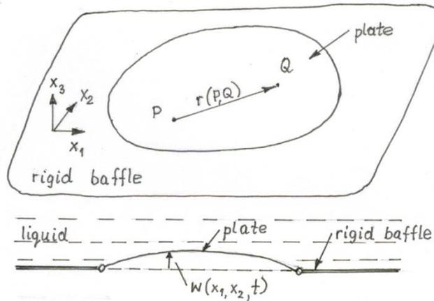
Figure 1. A plate in contact with liquid
