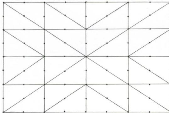
Figure 4. The discretization of a rectangular plate
