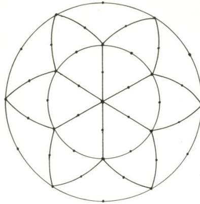
Figure 3. The discretization of a circular plate
