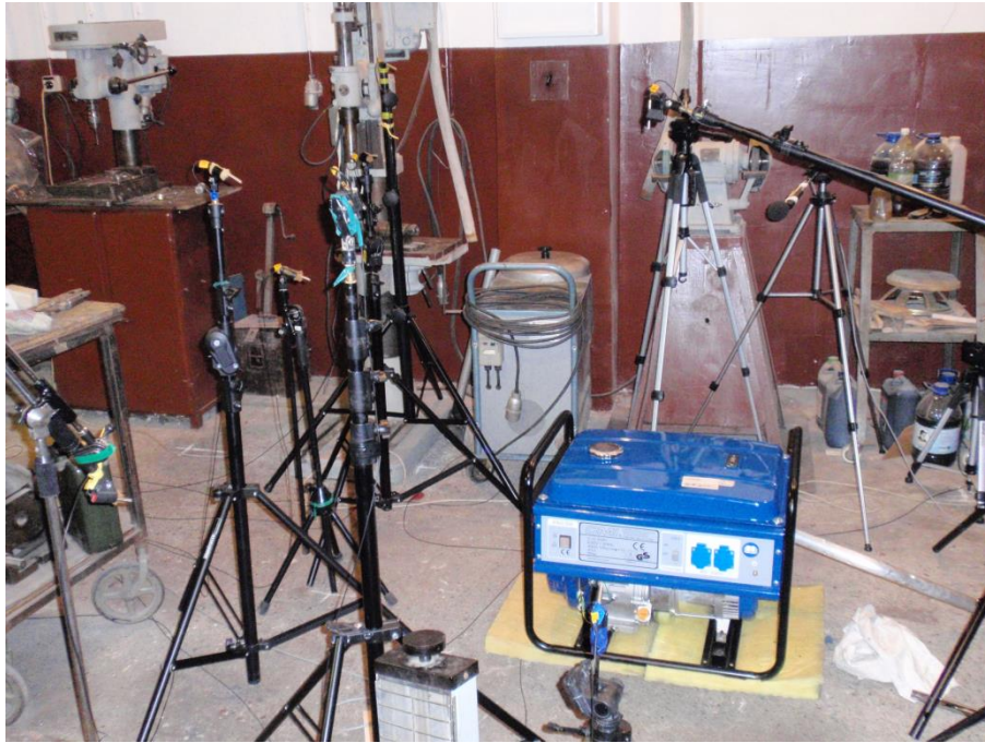
Fig. 3. Measurement of noise in the mechanical workshop using 12 microphones.
