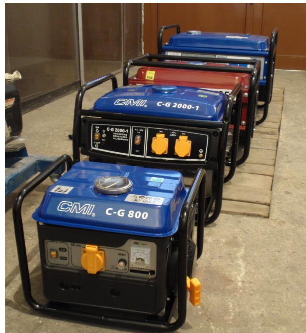
Fig. 1. Series of AC generators ready to test.
