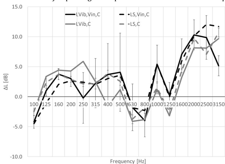
**Fig. 3.** The influence of the measured parameter (S – sound, Vib – vibration) and an additional layer of vinyl (Vin) on  $\Delta L$  results. Standard deviation given for  $L_{Vib,Vin,C}$  and  $L_{S,C}$  only.
