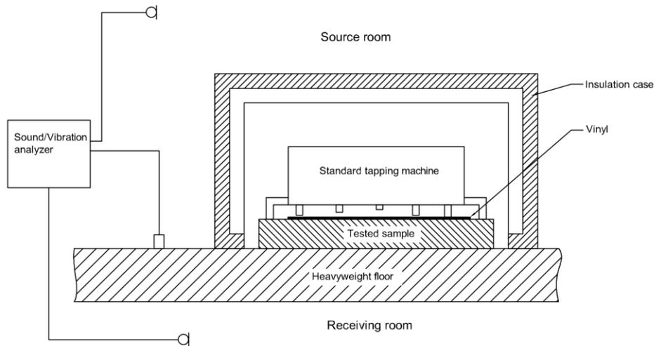
**Fig. 1.** Setup for the improvement of the sound insulation  $\Delta L$  measurement. The vinyl layer marked in the figure was used in selected measurements (Vin subscript in Tab.1.). The accelerometer and microphone were placed in six different positions (microphone in the source or receiving room).
