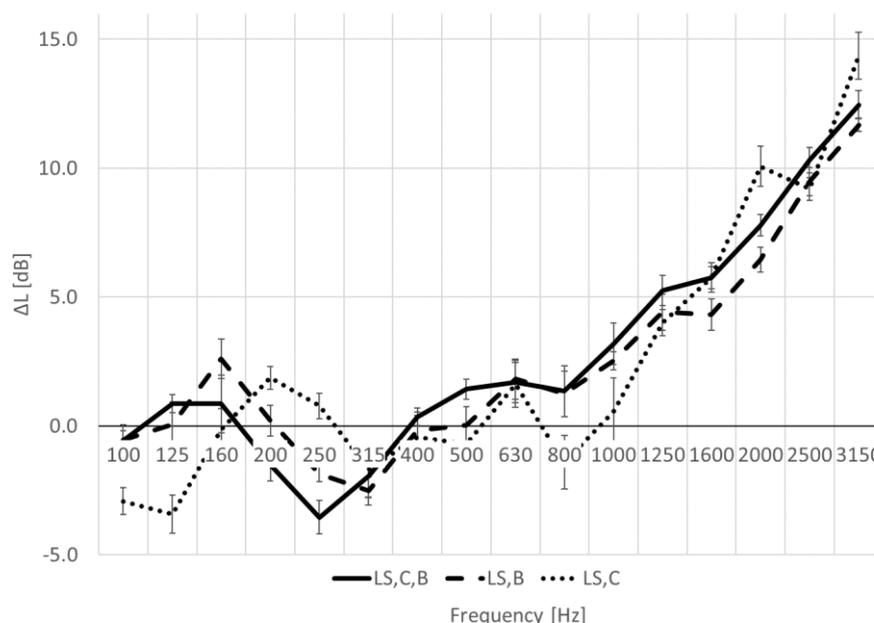
**Fig. 2.** The influence of the insulation case and receiving room localization on  $\Delta L$  results (with standard deviation). Measured parameter:  $L_{eq}$ . Solid line – with the insulation case, measured in receiving room, dash – without the case, measured in the receiving room, dotted – with the case, measured in the source room.
