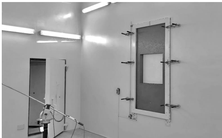
Fig. 1. View of the receiving room along with the measuring hole in the laboratory at AGH University of Science and Technology in Cracow.
