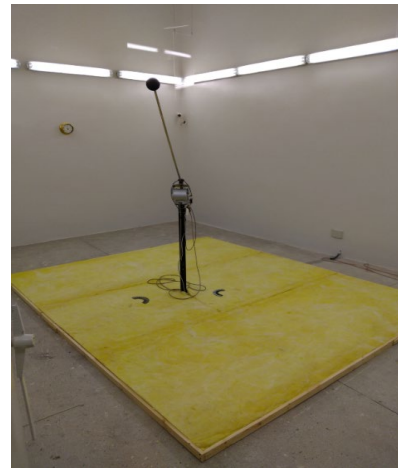
Figure 3. Reverberation chamber A. Sample - Isover Super Mata+ 50 mm.
