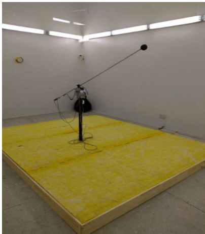
Figure 2. Reverberation chamber A. Sample - Isover Super Mata+ 150 mm.
