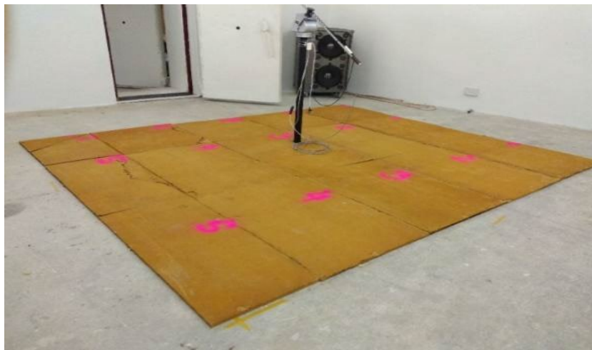
Figure 1. Reverberation chamber B. Sample - Fiberboard 20mm.
