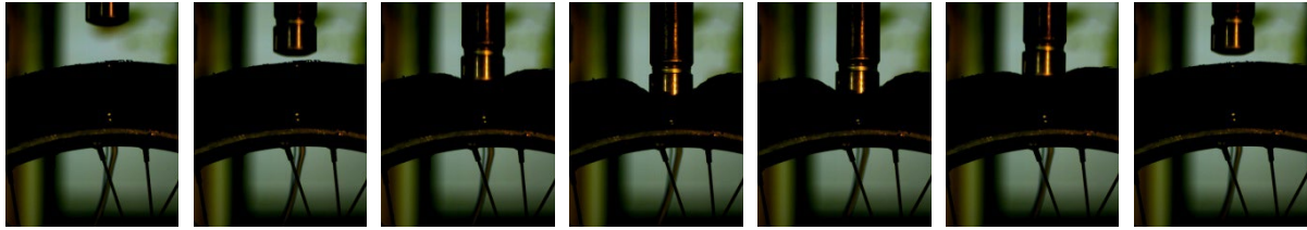
Figure 3. The stages showing the reaction of the tire on impact at a pressure of 1.8 bar, drop height of 0.6 m.
