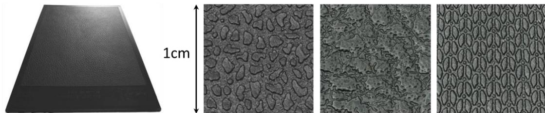
**Figure 5.** Example of test plate (21x15 cm) and microscopic view of texture 1 – 3 (from left to right)
