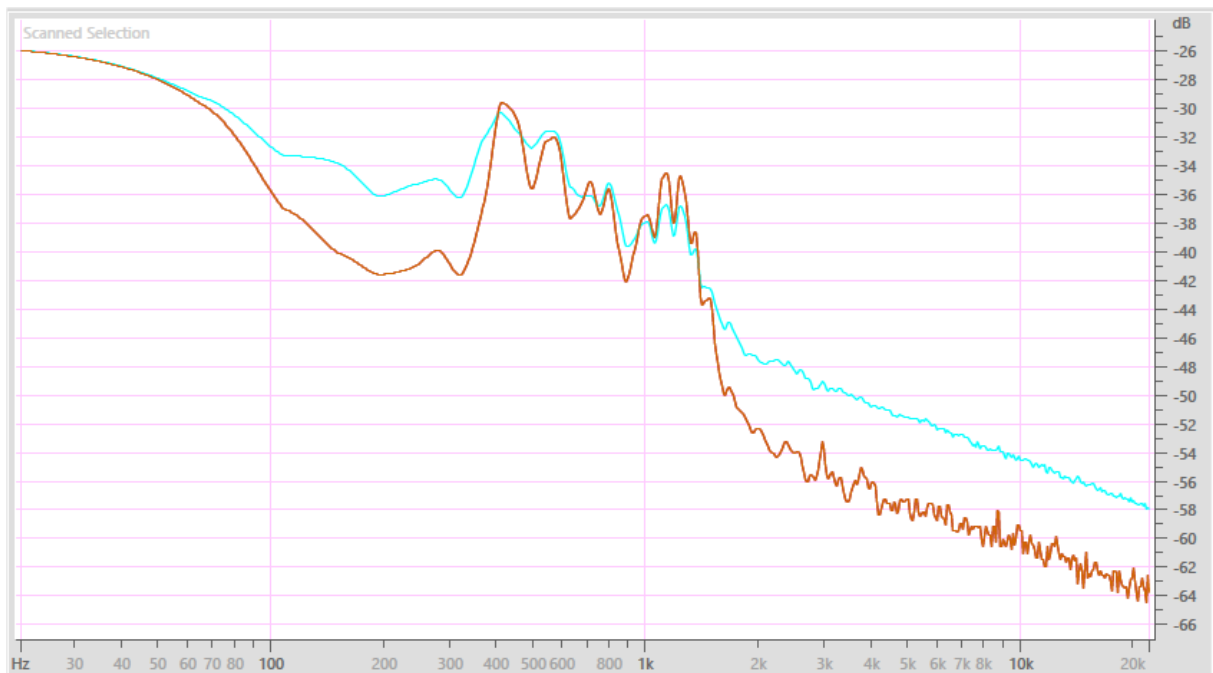
Figure 6. Comparison of the signal with noise before (blue) and after (red) the spectral denoising algorithm. Change of SNR was around +5 dB.
