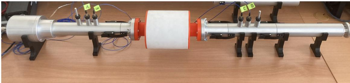
**Figure 1.** Measurement stand for testing acoustic mufflers.
