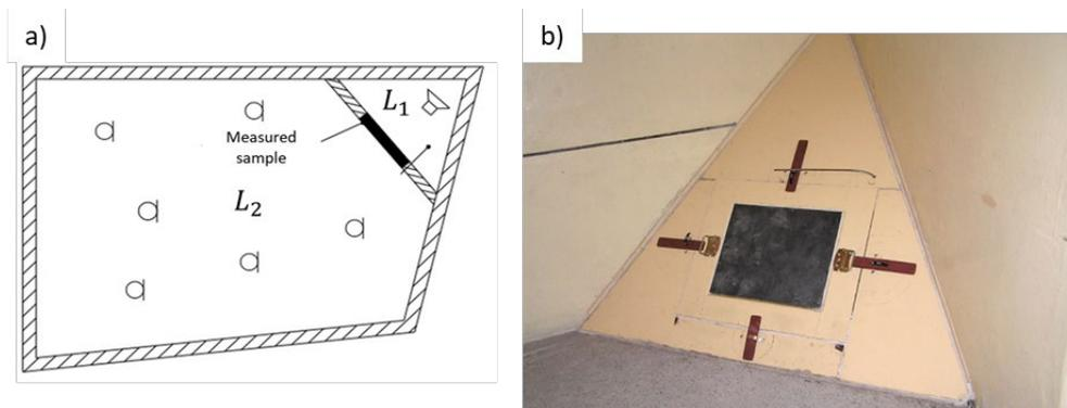
**Figure 2.** Scheme of the measurement setup with sound source, microphones and measured sample (a) and a photo of the measured sample in the reverberation chamber (b).
