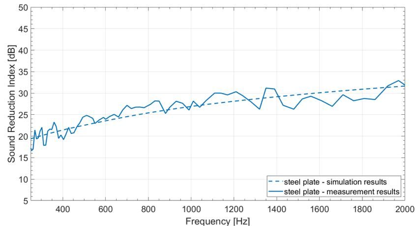
**Figure 4.** Simulation (dashed line) and measurement (solid line) results comparison for steel plain plate.
