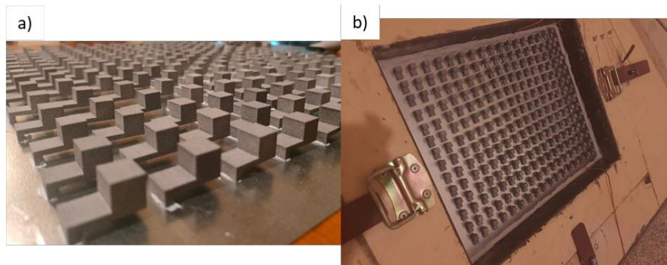
**Figure 3.** Photo of the steel plate with attached metamaterial structures (a) and sample placed in measurement window in the reverberation chamber (b).
