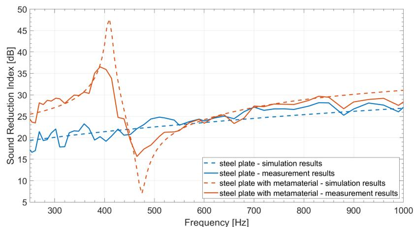
**Figure 5.** Comparison of the simulation and measurement results for steel plain plate (blue lines) and the same steel plate with metamaterial (red lines).
