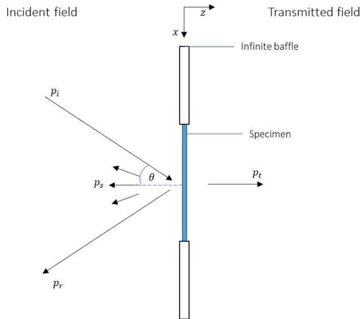
**Figure 1.** The model of finite sample in the infinite baffle with acoustic field on left and right side.
