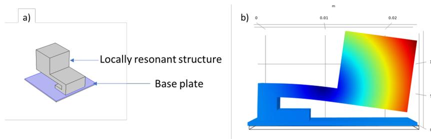
**Figure 1.** Comsol model of the unit cell with base plate and resonant structure (a). The excitation plane is marked with blue color. Mode shape of the first natural frequency of modeled structure (b).
